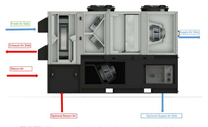
In ECRH ENERGY with heat recovery and economizer dampers, heat recovery and thermodynamics heat recovery are performed by the return fan. Some of the exhaust air is passed through the rotary type heat recovery unit according to the mixing ratio. Then, the heat transferred air is passed over the condenser coil directly. In this way, energy saving is achieved by thermodynamics heat recovery.
